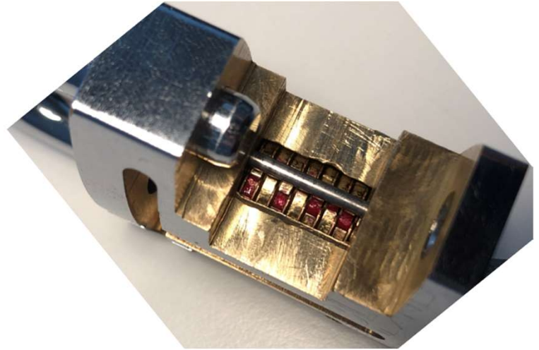
Paint added into each true gate for better visualization of picking status
