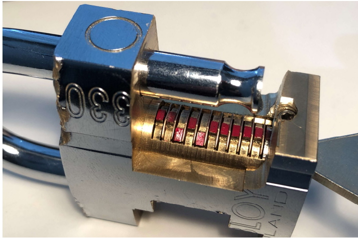
Paint added into each disc for better visualization of picking status
