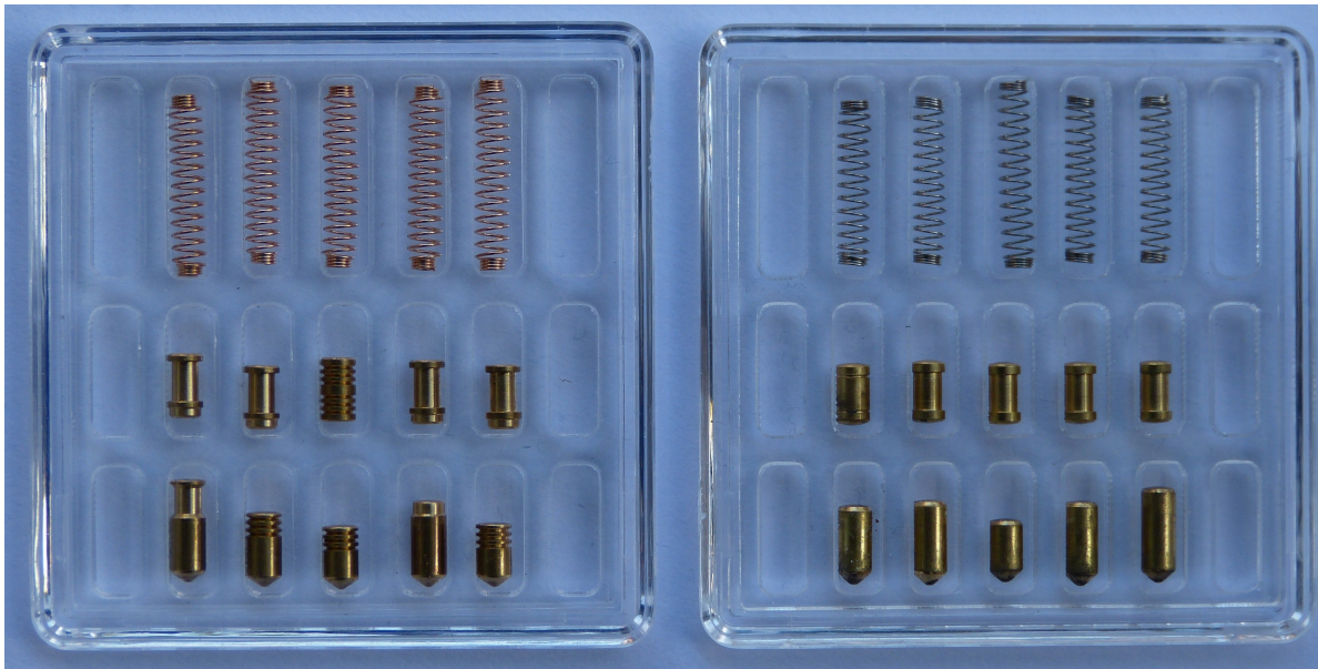
Figure 4: Reference set of pins. New pins on the left, and old pins on the right.
